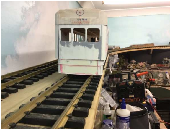
The sub floor Valance and 'Cow Catcher' were made and attached.
