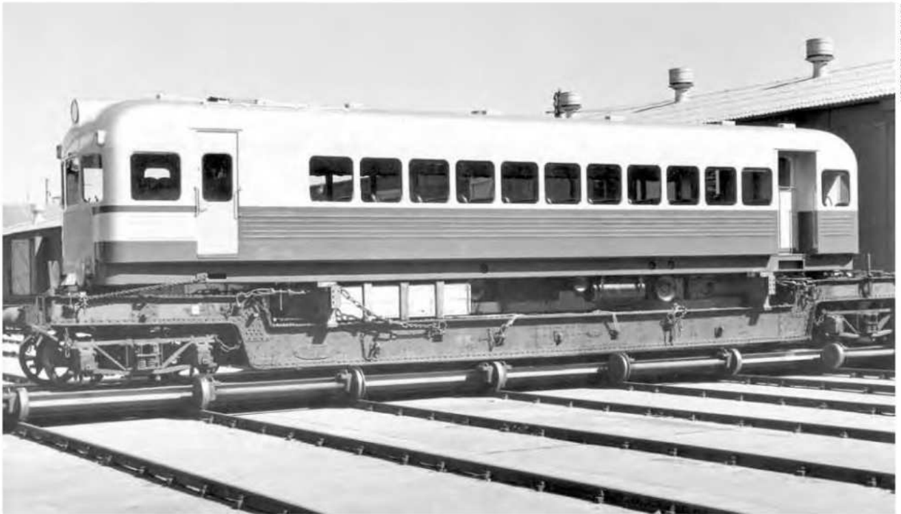
Completed 1800 class railcar (minus bogies) mounted on NSWGR well wagon in preparation for delivery to Queensland.
