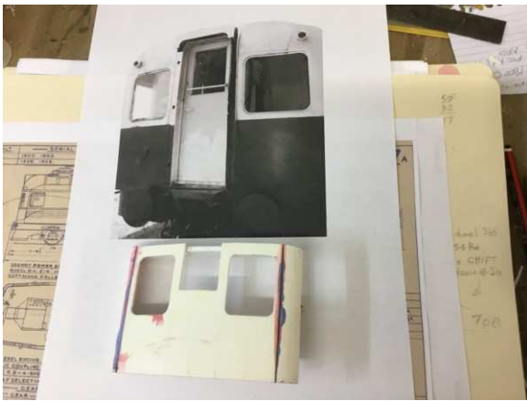
Back end wall, curved and stiffened with profile cut sill & forehead pieces.
