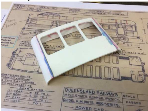
Front end wall, curved and stiffened with profile cut console & forehead pieces.
