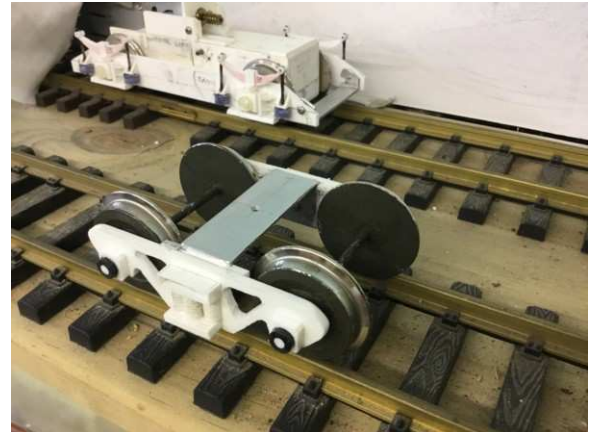
Bolster is 2.5mm Aluminium, bushings are bronze.
