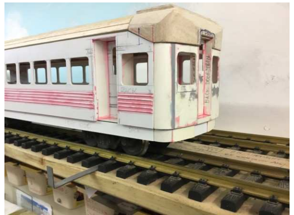
A lot of shaping and sanding yet of the roof. Brow / Forehead, mid roof is strips of balsa to be filled & sanded.
