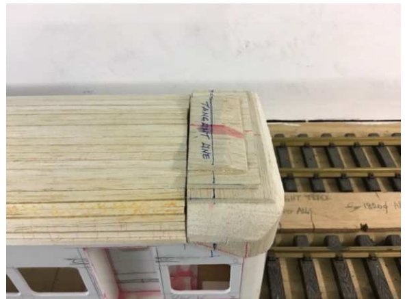
A lot of shaping and sanding yet of the roof. Brow / Forehead, mid roof is strips of balsa to be filled & sanded.
