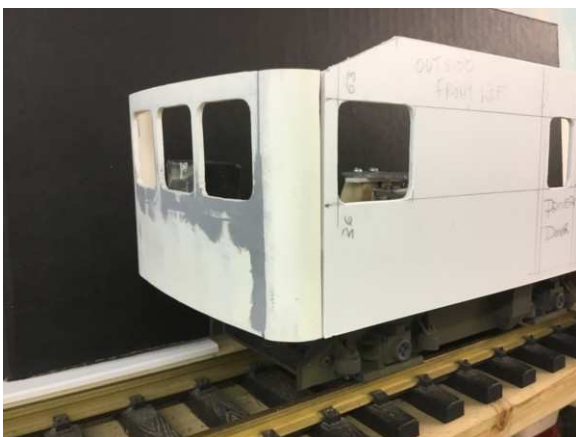
Photo of a check of alignment at corner joint.
