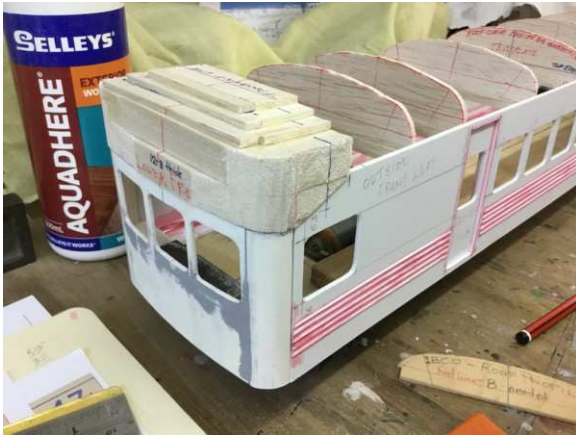
The front end layers of balsa ready for shaping.
