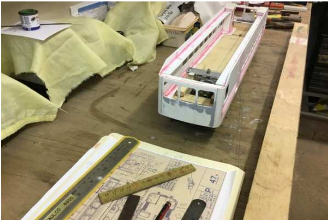
Now ready to start roof assembly. To keep centre of gravity low, roof is to be Balsa construction.
