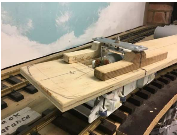
Testing clearances on 3'-0" radius curve.
