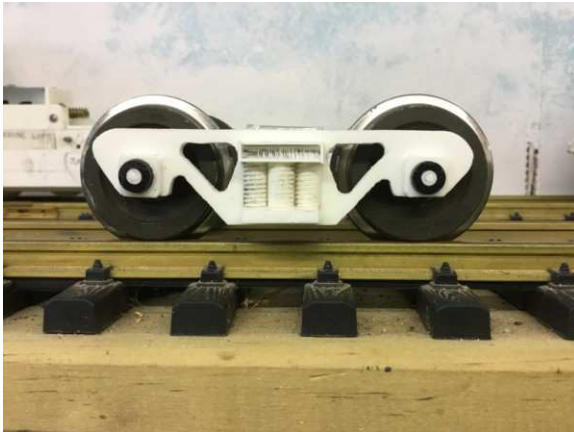
Side Frames were fretted from 3mm styrene,
