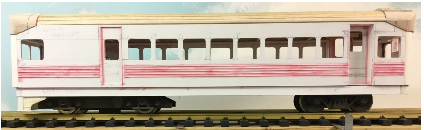
The sub floor Valance and 'Cow Catcher' were made and attached.
