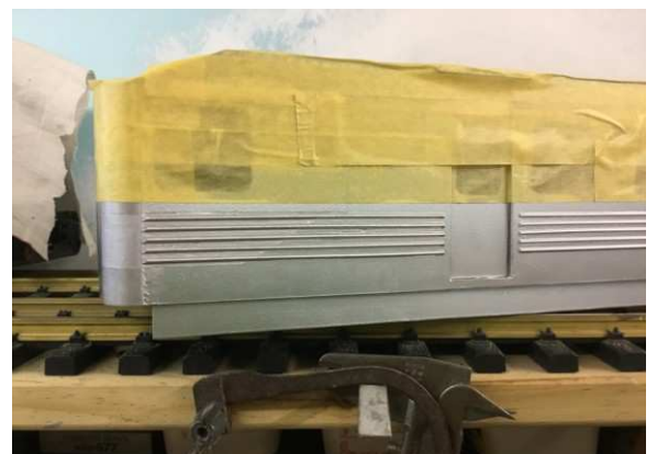
PVA glue used as a mask for curves & sweeps.
