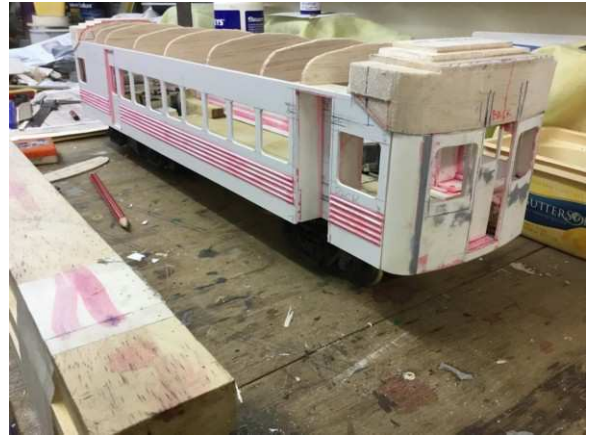
The back end balsa block prior to shaping.
